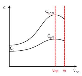
Initial capacitance C<sub>0</sub>: is the value at the origin of the hysteresis without any applied direct
